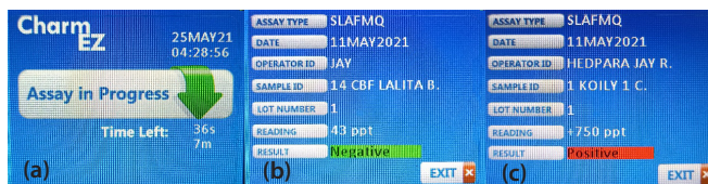
Plate 1: (a) LFA test display shows actual time to complete the test (b) Negative sample result found in the test (c) Positive sample found in the test along with reading of concentration of AFM1
