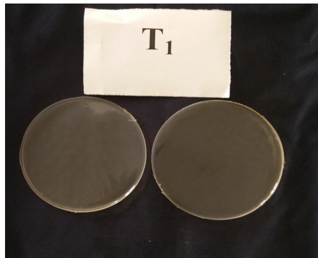
Fig. 6 Alginate films obtained with different concentrations of immobilized lysozyme
