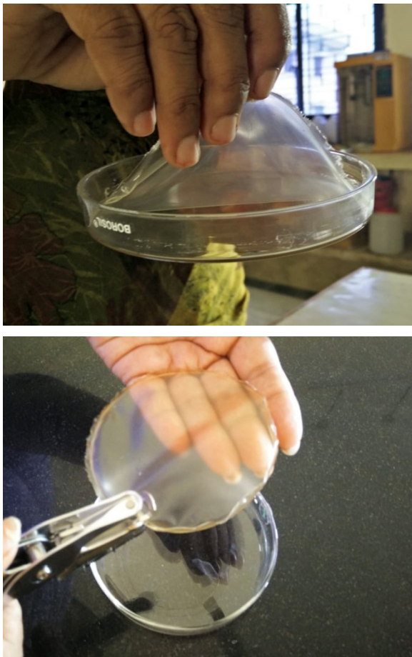
Fig. 3&4 Preparation of alginate films using petri plates
