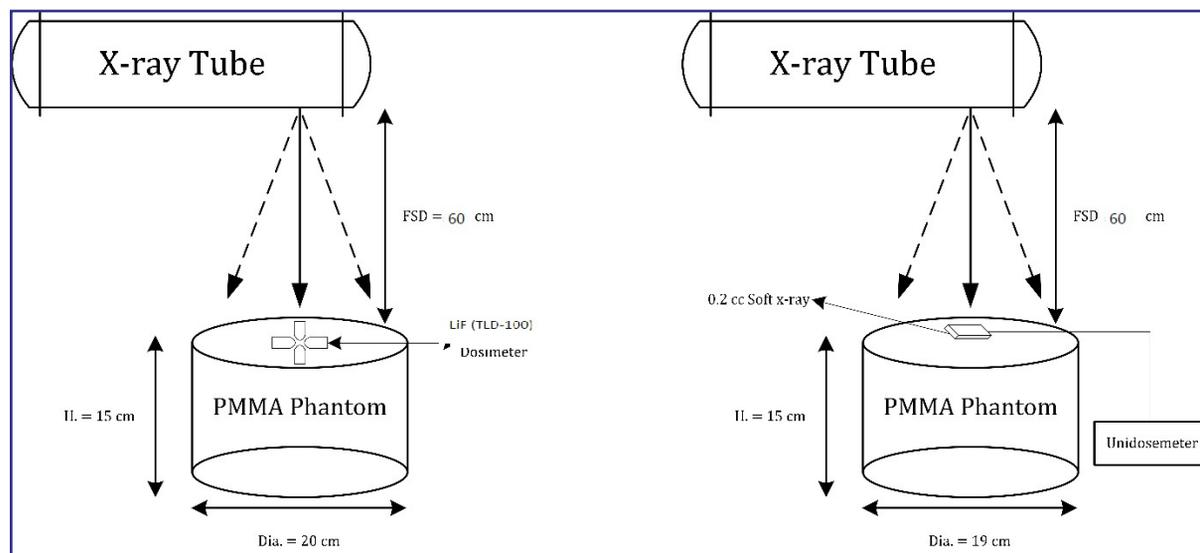
Fig. (1): The experimental arrangement for TLD dosimeter calibration.
