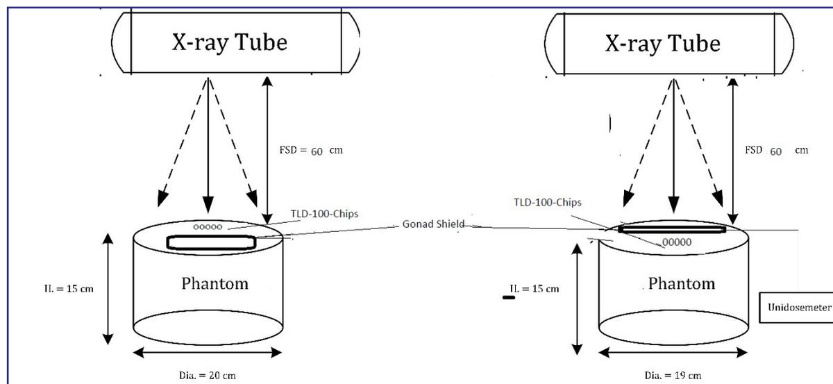
Fig. (2): The experimental arrangement for TLD dosimeter above and under gonad shield.
