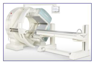
of the two cameras are listed in Table 1. It includes a removable Low Energy High Resolution (LEHR) lead collimator, Sodium Iodide doped with Thallium (NaI(TI)) scintillation crystal, a light guide and 59 photomultiplier tubes (PMTs). The LEHR collimator features parallel holes with hexagonal patterns and is used for low energy sources such as Tc-99m.
