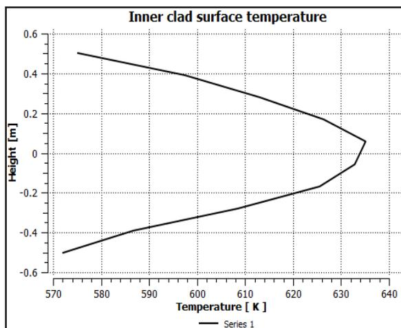
Fig. (5):  $(Th_{0.9}U_{0.1}) O_2$  annular fuel Inner clad surface temperature along the height.
