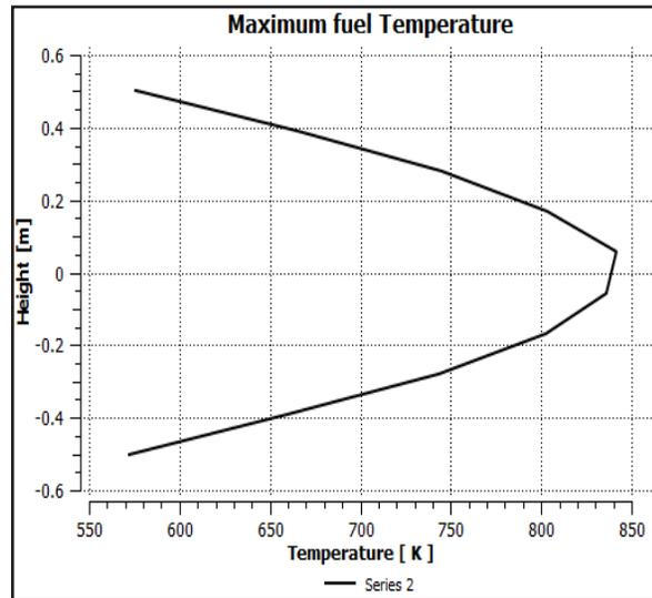
Fig. (6):  $(Th_{0.9}U_{0.1}) O_2$  annular fuel temperature at 5.25 mm axial line from the center along the height.
