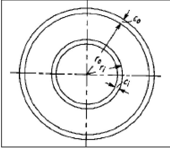
Fig. (3): Annular fuel element with inner and outer clad .
