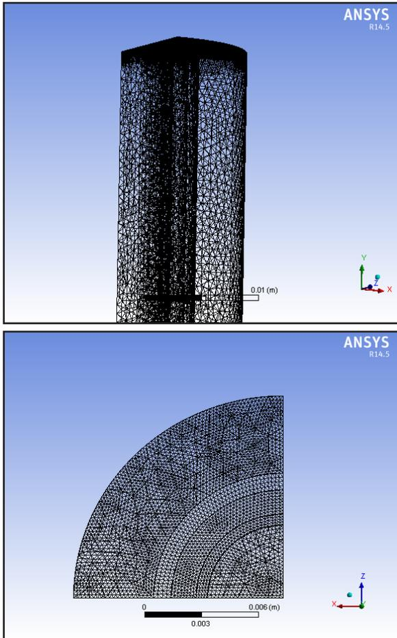
Fig. (2): The finite element equivalent cell model for the dual cooled proposed fuel.
