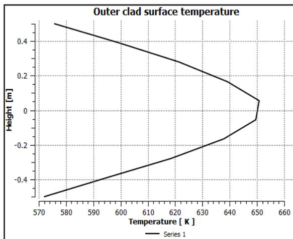
Fig. (4):  $(Th_{0.9}U_{0.1}) O_2$  annular fuel outer clad surface temperature along the height.
