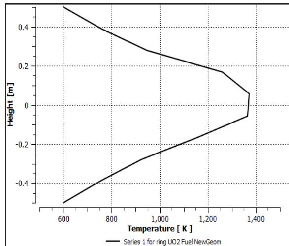
Fig. (7): Conventional  $UO_2$  Fuel temperature at 1.517 mm axial line from the center along the height.
