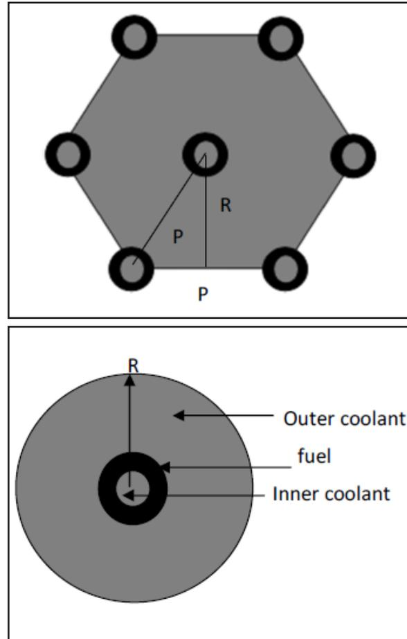
Fig. (1): The equivalent cell.
