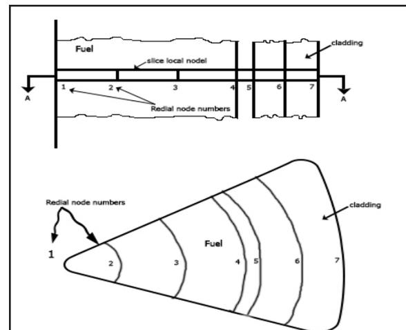
Fig. (1): Radial fuel rod discretisation.
