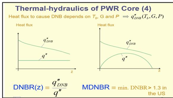
Fig. (2): Typical relation shapes of heat flux and  $\bar{q}''_{DNB}$  distribution along the fuel axis.
