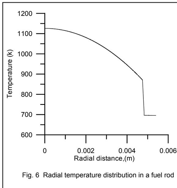
Fig. 6 Radial temperature distribution in a fuel rod
