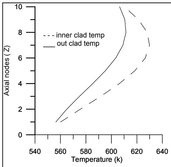
Fig. 5 Internal and external clad temperature (k)
