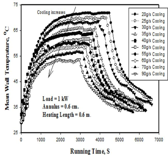
Figure (2): Theoretical worm-up, stable-state and cool-down of mean evaporator wall temperature for sub-cooled heat-pipe at variable cooling rate.
