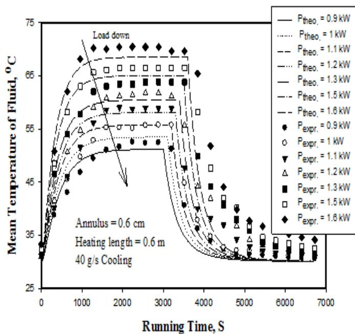
Figure (8): Investigate warm-up, and cool-down under stable state of mean fluid temperature for sub-cooled heat-pipe at variable loads of heating.
