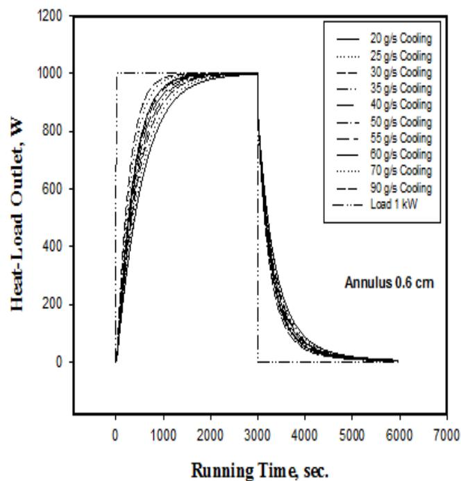
Figure (10): Theoretical power output for sub-cooled heat-pipe during warm-up, stable-state and cool-down at annulus 6mm and Power 1 kW variable coolant-rates.
