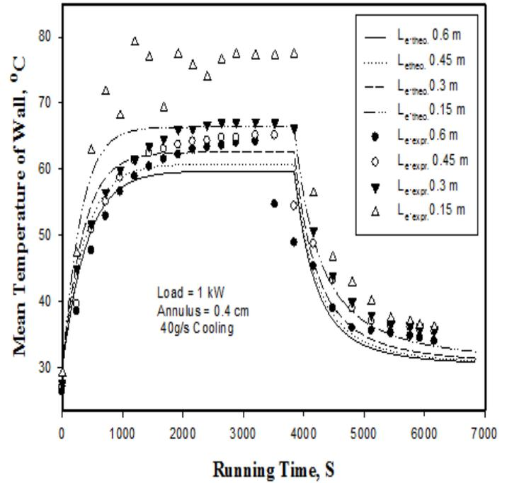
Figure (5): Experimental and theoretical worm-up, stable-state and cool-down of mean evaporator wall temperature for sub-cooled heat-pipe at variable evaporator lengths.
