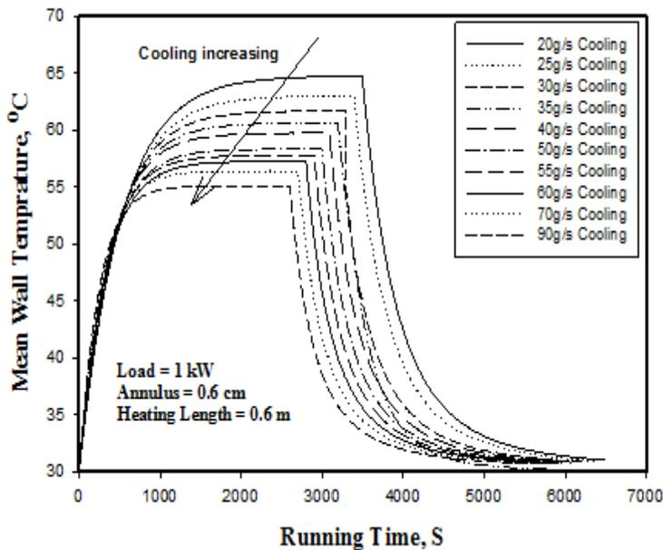
Figure (3): Experimental worm-up, stable-state and cool-down of mean evaporator wall temperature for sub-cooled heat-pipe at variable cooling rate.
