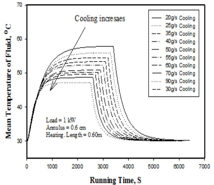
Figure (6): Theoretical warm-up, stable-state and cool-down of mean fluid temperature for sub-cooled heat-pipe at variable cooling rate.
