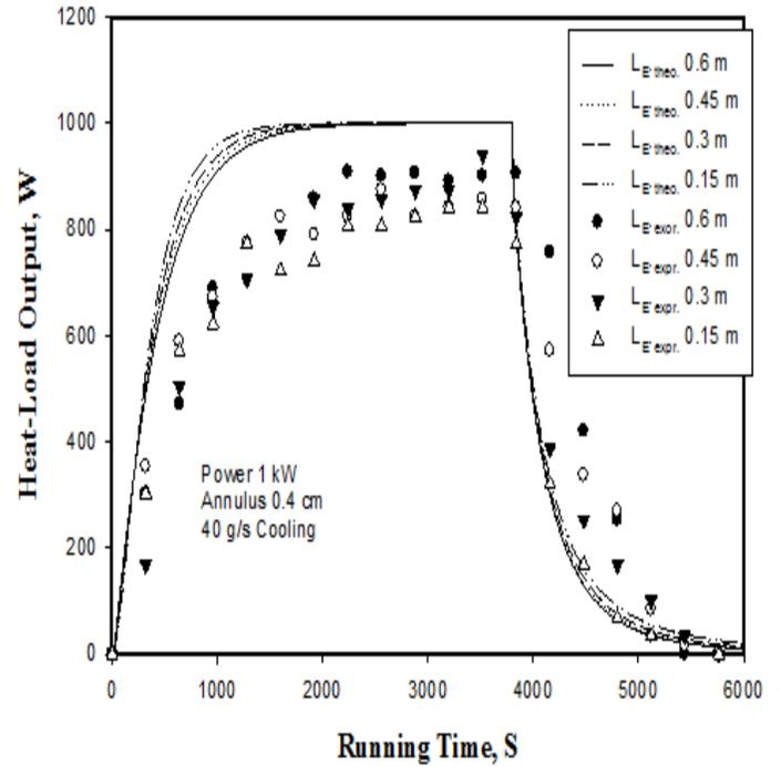
Figure (13): Experimental power output for sub-cooled heat-pipe during warm-up, stable-state and cool-down at variable evaporator lengths.
