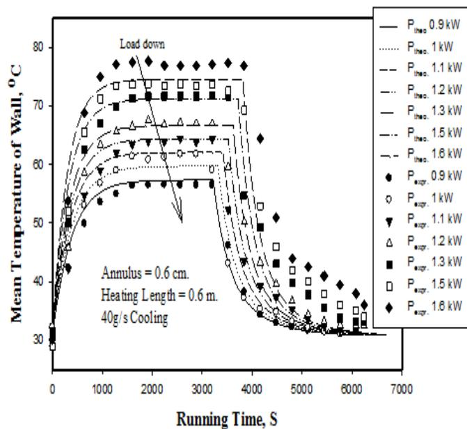
Figure (4): Theoretical and experimental worm-up, stable-state and cool-down of mean evaporator wall temperature for sub-cooled heat-pipe at variable heat-loads.
