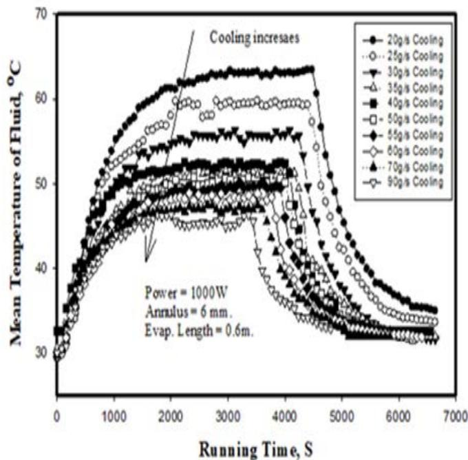
Figure(7) Experimental warm-up, stable-state and cool-down of mean fluid temperature for sub-cooled heat-pipe at variable cooling rate.
