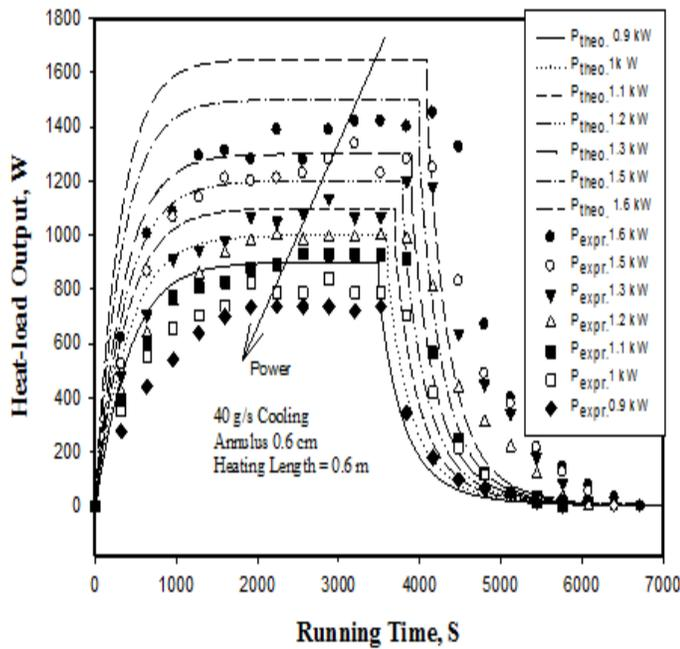
Figure (12): Experimental power output for sub-cooled heat-pipe during warm-up, stable-state and cool down at variable power in-put.
