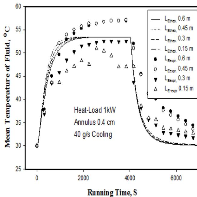
Figure (9): Experimental and theoretical warm-up, stable-state and cool-down of mean fluid temperature for sub-cooled heat-pipe at variable evaporator-lengths.
