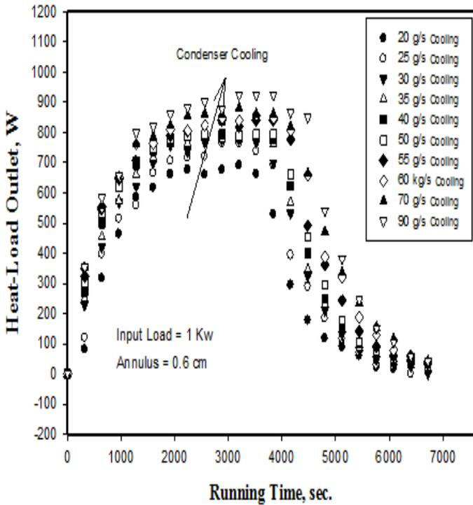
Figure (11): Experimental power output for sub-cooled heat-pipe during warm-up, stable-state and cool-down at variable coolant-rates.
