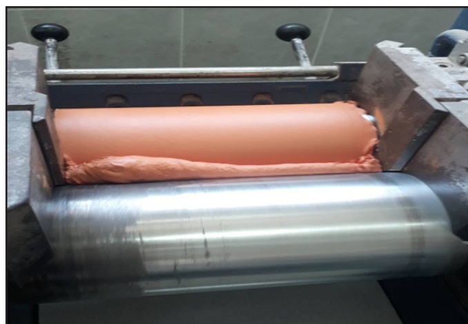
Figure (1): Uniformly mixed composite sample in a two-roll mixer
